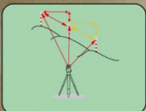
Missing line measurement
